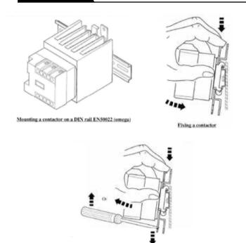
Removing a contactor by hand or with a screwdriver
