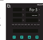
Display Previous Fault Output 3
